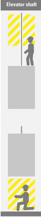
Before entering the shaft with reduced shaft head / pit acc. to EN 81-21, the **Shield Mode Maintenance** will be activated via the door release. A refuge space that enables safe working for the maintenance employees is created.
