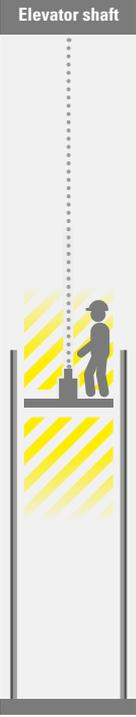
**Shield Mode Installation** ensures a refuge space for the employees even before the elevator is put into operation. During scaffoldless installation, such as rail fastening, a refuge space is created sequentially according to the progress of the installation. Depending on the position, the car is secured with a tolerance of  $\pm 5$  cm.
