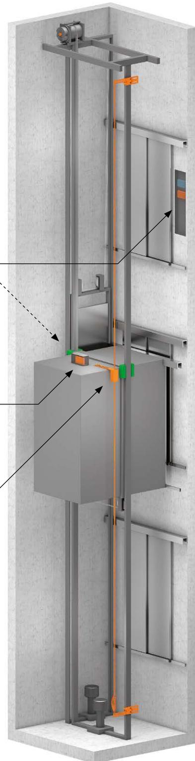
This allows functions such as emergency limit switches, delay control, door override or inspection switches to be implemented in the case of a shortened shaft head or shaft pit in accordance with EN 81-21. The avoidance of unintentional car movements (UCM) as well as the installation of refuge spaces for assembly and maintenance are also possible.
