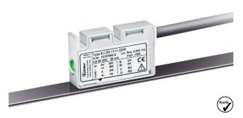
The non-contact incremental magnetic linear measurement system Limes LI20 / B1 - made up of the sensor head LI20 and of the magnetic band B1 - reaches a resolution up to 10 µm with a maximum distance of 1 mm between the sensor and the band.
