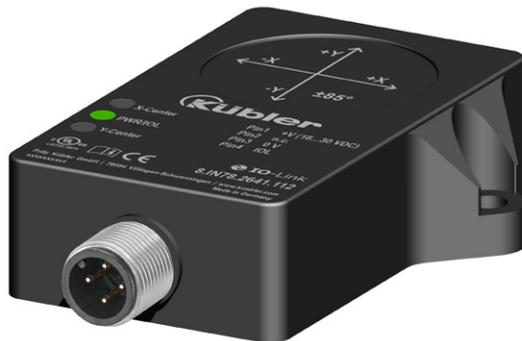
The inclinometers of the IN78 series are used to determine 2-axis inclinations in the measuring range of  $\pm 85^\circ$  or 1-axis inclinations up to  $360^\circ$  via a sensor fusion of acceleration and rotation rate measuring cell (gyroscope). Various parameters can be customized for individual requirements (e.g. via the PACTware software). Thanks to their high robustness, the inclinometers are also ideally suited for outdoor use.
