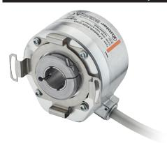
The optical Sendix F5883 multiturn encoder in the Motor-Line version stands out particularly because of its reduced overall depth of only 43 mm with a through hollow shaft up to 15 mm.
