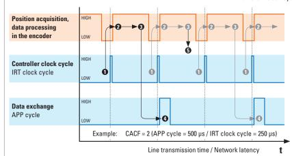
IRT clock cycle = Transmit clock
