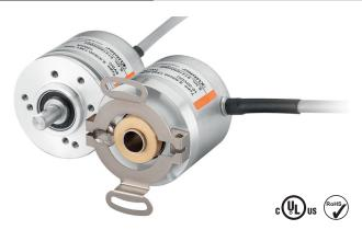
The incremental encoders type Sendix Base KIS40 / KIH40 with optical sensor technology have been designed for highest cost-effectiveness. They are available with a resolution of up to 2560 pulses per revolution.
